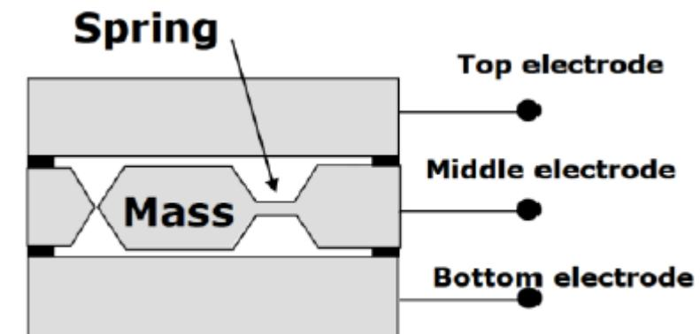
Q2.10: Tilting MEMS at SAFRAN-Colibrys operating at 175°C, provide the application ?
