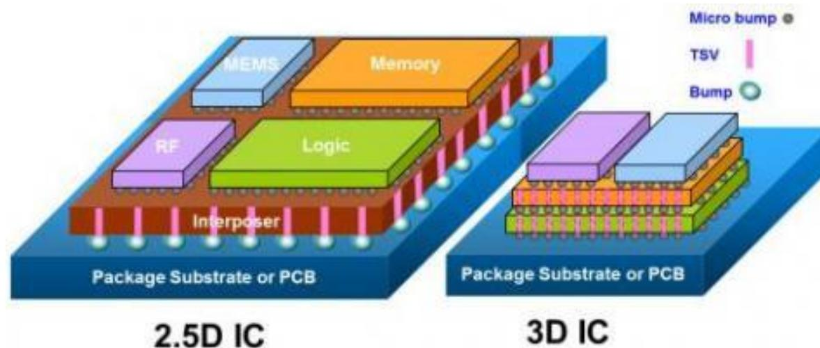
3D: Through Silicon Vias (TSVs) made directly in the functional substrate(s)
